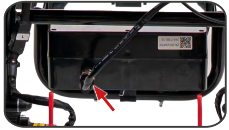
Illustration 8. Connecting the battery power connector.
