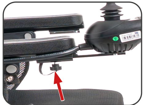
Illustration 12. Control panel adjustment screw.
