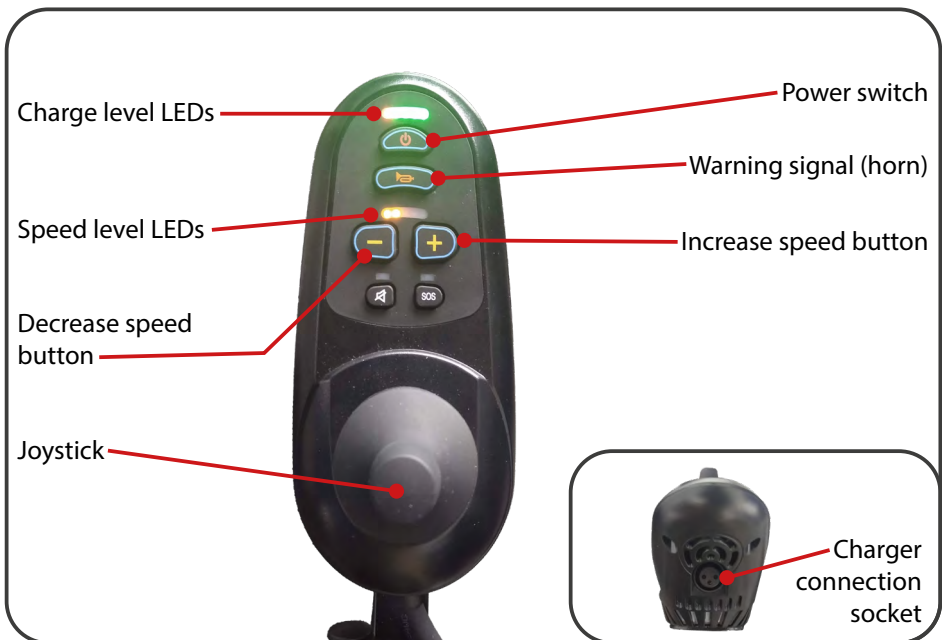
Illustration 3. Control panel (joystick)
