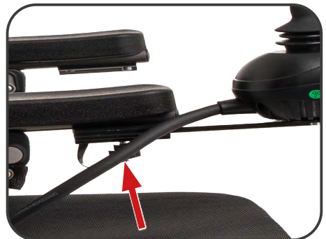
Illustration 12. Control panel adjustment screw.
