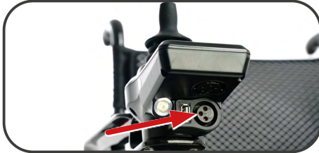
Illustration 16. Connecting the charger to the controller.
