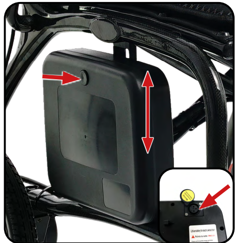
Illustration 11. Disconnecting the battery and charging outside the wheelchair.
