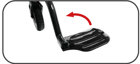
Illustration 9. Folding frame and foot-rests.
