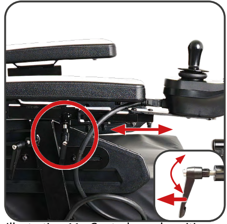
Illustration 11. Control panel position adjustment.
