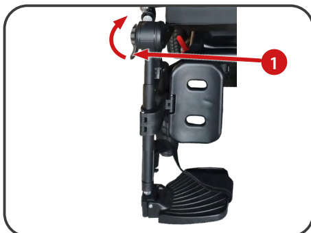
Illustration 15. Adjustment of the angle of the footrests.
