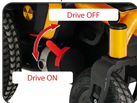
Illustration 4. Location of the drive disconnect lever.
