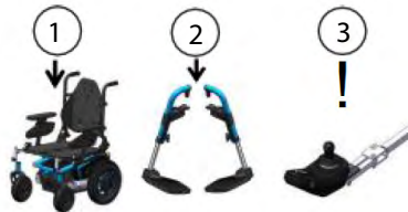
Illustration 14. Removal of wheelchair components.
