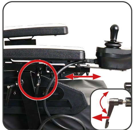
Illustration 7. Control panel position adjustment.
