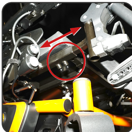
Illustration 14. Footrest position adjustment.
