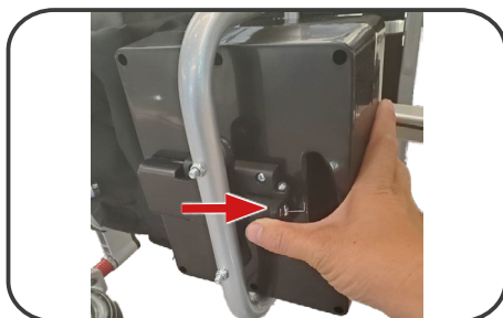
Illustration 9. Battery installation and removal.
