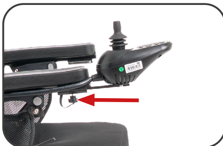
Illustration 6. Controller installation.
