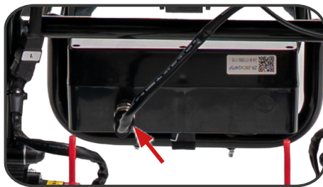
Illustration 8. Connecting the battery power connector.
