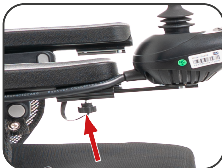
Illustration 12. Control panel adjustment screw.
