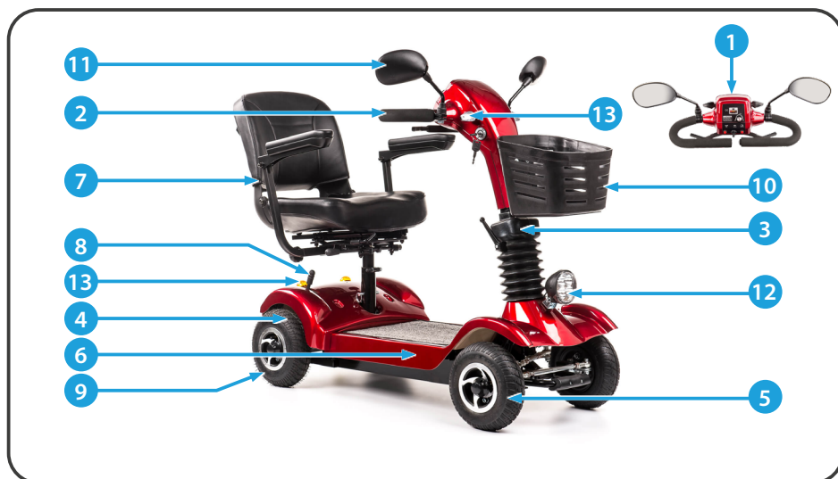
Illustration 1. List of MINI wheelchair components.
