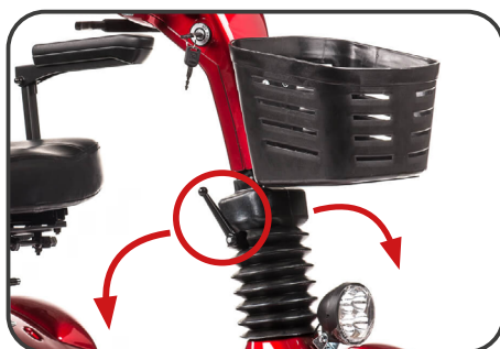
Illustration 3. Steering column angle adjustment.
