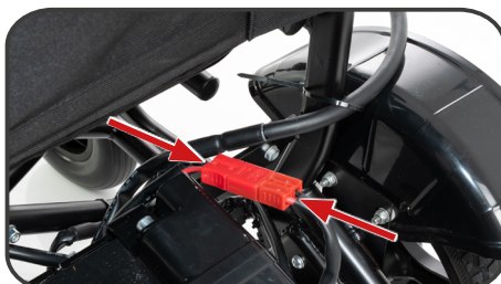
Illustration 7. Connecting the battery power connector.
