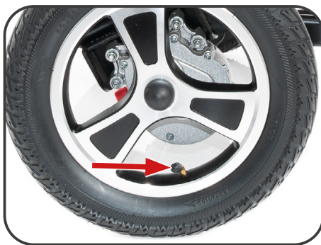
Illustration 26. "Schrader" valve (car valve)
