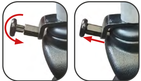
Illustration 24. Front wheel lock.
