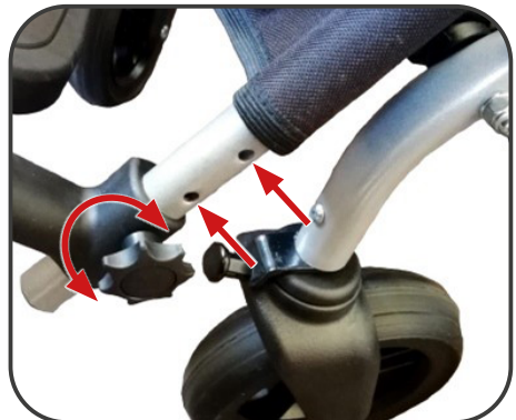
Illustration 16. Footrest length adjustment.
