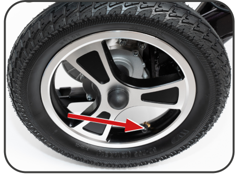
Illustration 22. "Schrader" valve (car valve)
