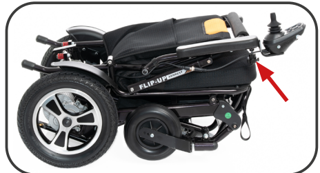
Illustration 5. Control panel adjustment screw.
