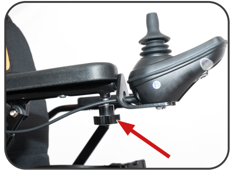
Illustration 9. Control panel adjustment screw.
