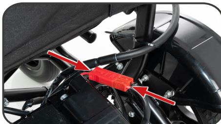
Illustration 7. Connecting the battery power connector.
