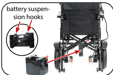
Illustration 6. Install battery.
