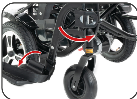
Illustration 9. Installation of the footrest.
