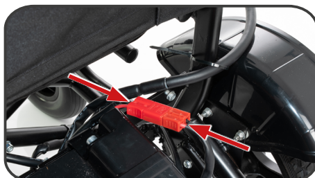
Illustration 7. Connecting the battery power connector.
