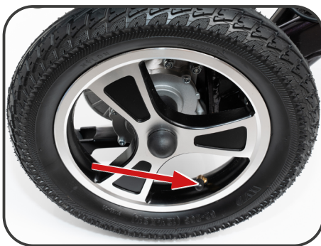
Illustration 22. "Schrader" valve (car valve)
