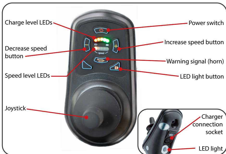
Illustration 3. Control panel (joystick)
