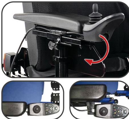
Illustration 8. Tilting the control panel control.
