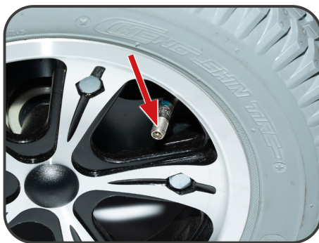
Illustration 16. "Schrader" valve (automotive)
