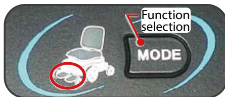
Illustration 12. Footrest tilt adjustment.
