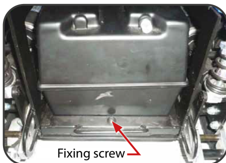
Illustration 4. Battery installation.
